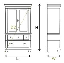
Case goods diagonal depth DD must be less than the entryway dimension 1, stairway dimensions 3, 4 & 8 and all interior doorways 6 or 7.
